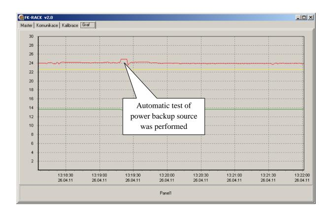
The chart shows graphically the status of power supply (mains) and power backup sources, including performed tests.
