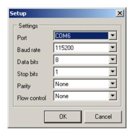
**Port** – enter the port number in the PC connected to the device. Leave other settings as predefined by the system unchanged. Settings are shown in the screenshot.
